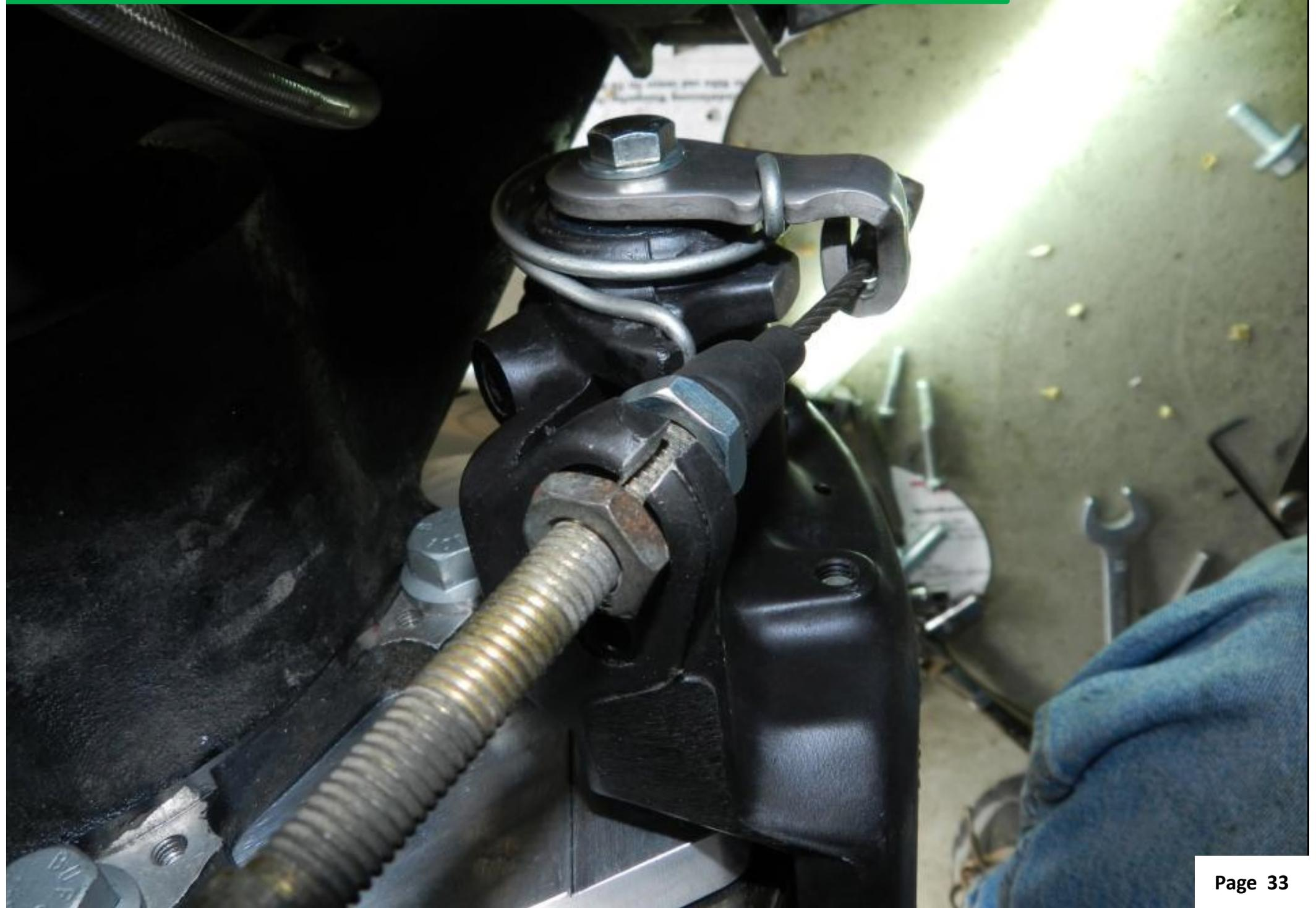
Detailed picture of caple attachment to caliper.
