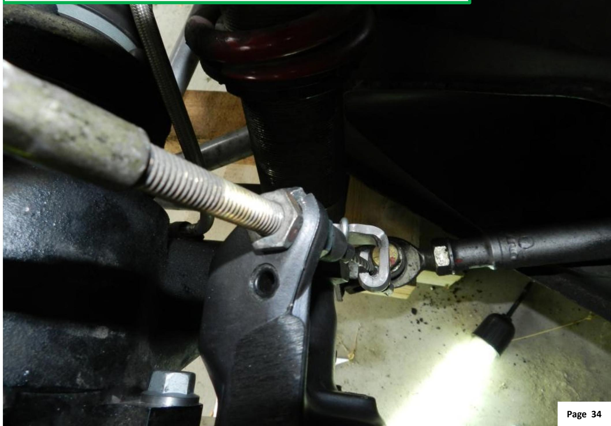
Detailed picture of caple attachment to caliper.
