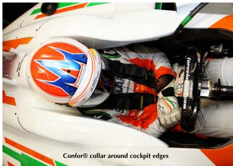
Confor® collar around cockpit edges
