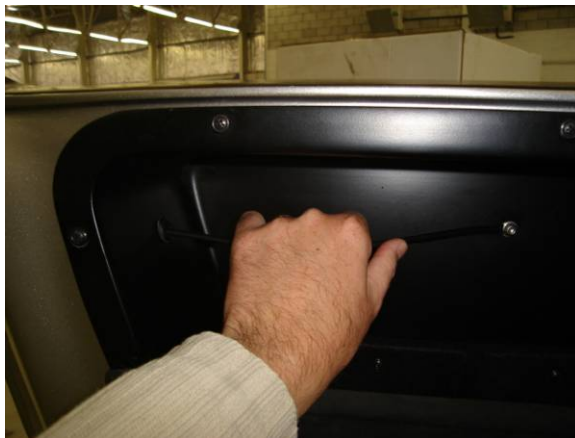
[Figure 6 – Opening the door from the inside]
