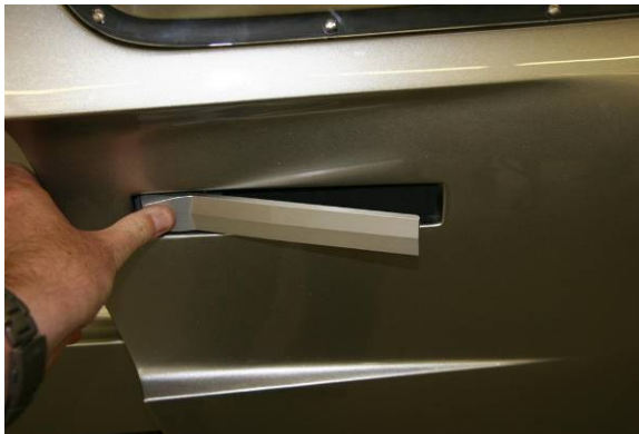
[Figure 5 – Opening the door from the outside]
