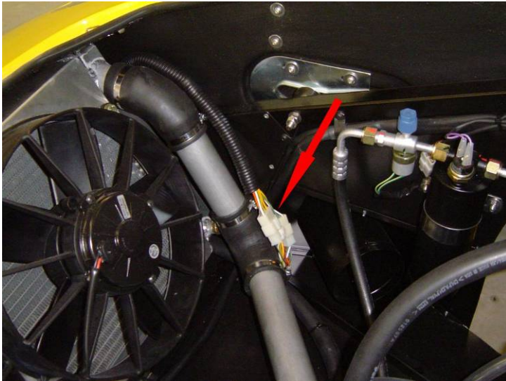
[Figure 9 – Headlight harness plug]
