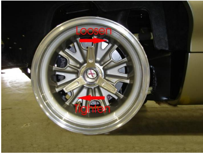
[Figure 17 – The right side front and rear wheel spinners are loosened by turning them clockwise and tightened by turning them counterclockwise.]
