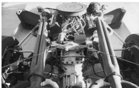
In the engine bay, most parts were specially fabricated or modified. I designed all components such as suspension, intake induction and exhaust headers. An unusual but needed adaptation was the use of an Offenhauser manifold and Holley carburetor to allow rearward visibility over the air cleaner. The headers were of a custom arrangement that provided an overhead exhaust flow. These items were built by certified machinists and welders, as I did not have the required skills.
