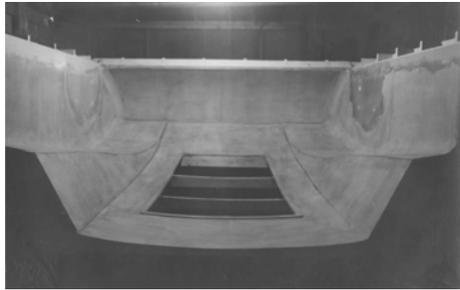
The bodywork was formed from fiber glass panels. "One-shot" female molds minimized total work and expense while producing smooth and continuous contours. Cross-sectional wooden frameworks were fabricated for the major body panels. Each framework was lined with sheetrock, which when wetted easily shaped into the contours. Finer detailing and a smooth finish were gained from tape and bedding compound. Finally, the molds were shellacked and waxed.
