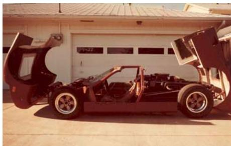
Due to the car's small size, components were packed together like a Chinese puzzle. Usually such a compact configuration would be difficult to maintain. To ease access for minor repairs and adjustments, the front and rear body panels were designed to swing clear of the chassis. Both panels can also be easily removed. This simplifies major repair efforts such as engine removal, which can be done in one hour.
