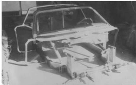
Chassis construction and the rear suspension used features not found in "street" cars. The chassis utilized three structural design types: Twin-tubes form the basic frame; the roll cage and scaffolds are space frame construction; and semi-monocoque panels act as stress members simultaneously forming walls. This hybrid structure provided a rugged yet light frame.
