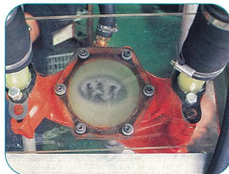
Pump and ancillary tests are performed on rig, and in this case steam vapour and air bubbles accumulate on pump low pressure point resulting in cavitation.
