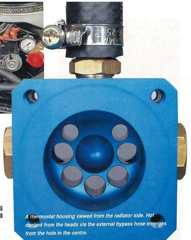
A thermostat housing viewed from the radiator side. Hot coolant from the heads via the external bypass hose emerges from the hole in the centre.
