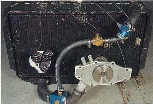
RIGHT: A de-aeration canister. The large connection at left is attached to the engine outlet. It has a nozzle inside it and its offset entry causes the coolant to swirl around the inside of the canister. The outlet at right is curved downward inside the canister so draws only fresh bubble-free coolant from the bottom of the unit. The small outlet at the bottom is the feed point for the external bypass hose.
