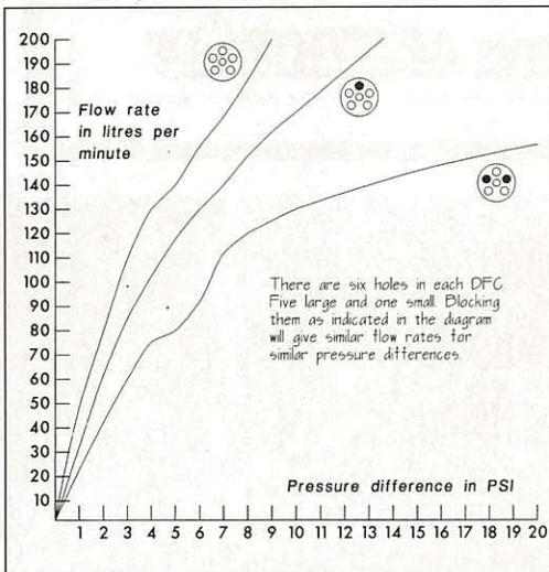
This rate must be slowed by restricting the flow. With an EcoTrans system, this is done by plugging a number of holes in the DFC. John calls this 'tuning the cooling system'. The DFC fitted to the 460 shown has six holes which have a total area of 0.794 square inches. As we mentioned, a healthy pump creating a pressure drop of 15psi across such a DFC creates a flow of 200 litres per minute (see graph). In the end, Wayne found that blocking two of the holes created the most effective flow rate.
