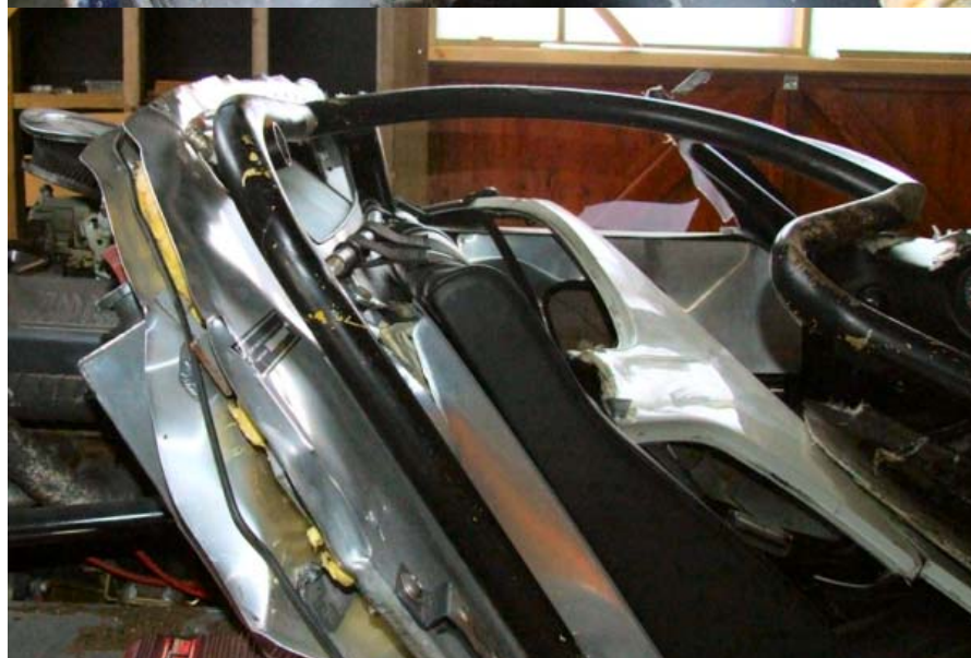
Massive distortion of the roll cage
