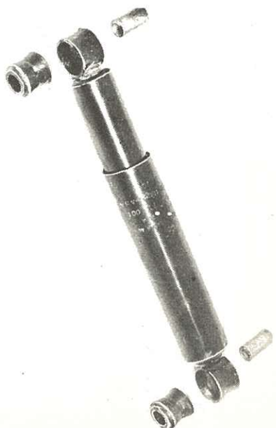
FIG. 29 — Shock Absorber Assembly
