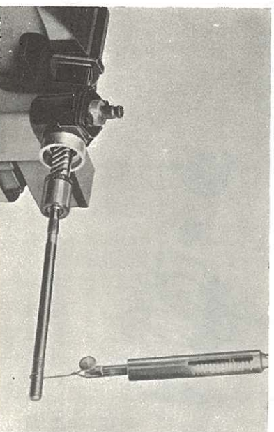
FIG. 6 — Tie Rod Pre-Load Check
