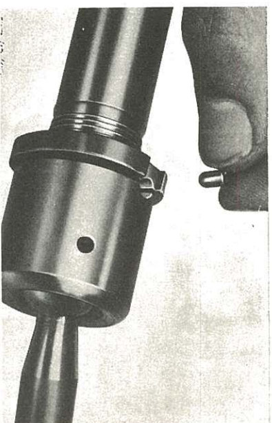
FIG. 8 — Fitting Retaining Pin
