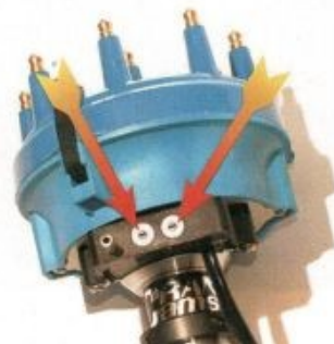
CRANE'S ALL-ELECTRONIC distributor has a combined total of 36 rpm and vacuum advance curves built in. These are selected by turning the two indicated screwdriver slots to a number corresponding to the curve required.
