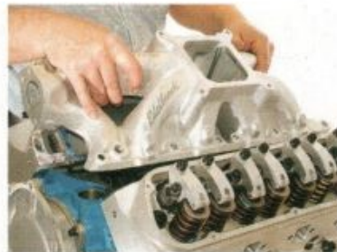
WE CHECKED out T&L's port-matching job and it proved to be right on the money both width-wise and top to bottom. The manifold was secured with stainless washers and 12-point bolts.
