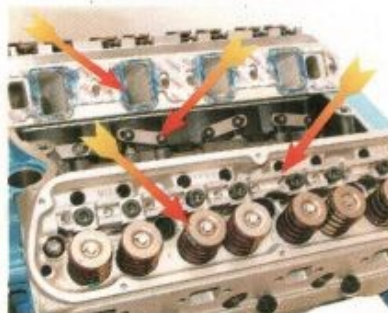
THERE ARE several points to note from this shot. First the manifold gaskets are preglued to the heads so they do not move when the manifold is installed. Second is that the lifters must be installed before the heads. Third, the arrow shows the pedestal for the Jesel rockers bolted in place. Lastly, note the titanium retainers, which hold the Isky "tool room" springs in place.
