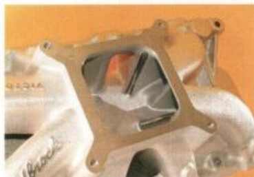
THE WORKMANSHIP on this T&L ported intake had to be seen in the flesh to be appreciated. The porting was not just cosmetic, but sought to achieve the best port tapers for the job.
