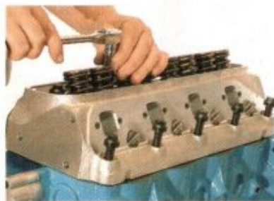
AFTER LOCATING the Fel-Pro head gaskets, the T&L ported Edelbrock Victor Jr. heads were bolted down using ARP's more friendly priced six-point bolts.
