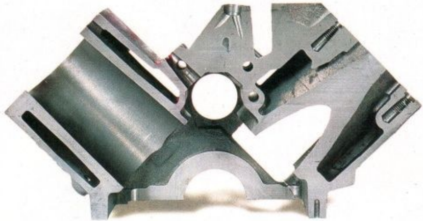
A PROMINENT feature of this sectioned Dart 302 iron Eagle block is its massive cylinder-wall thickness. Even with a 4.25-inch bore, the walls are still 10 percent thicker than a stock bore. Also worth noting are the blind head-bolt holes. That means no more rusty head bolts on teardown.
