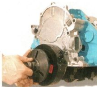
THE CRANK damper used was from Professional Products, and was conveniently marked with several degree scales. This allowed the use of any one of three different types of TDC pointers.
