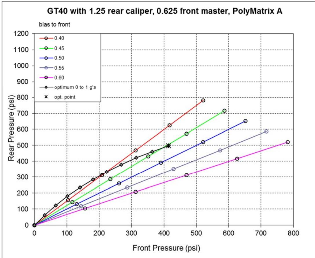
This graph shows that I can achieve 1.0 g's of braking at 70 pounds from the foot with 45% bias bar to the front. Now I can lock the tires easily.
