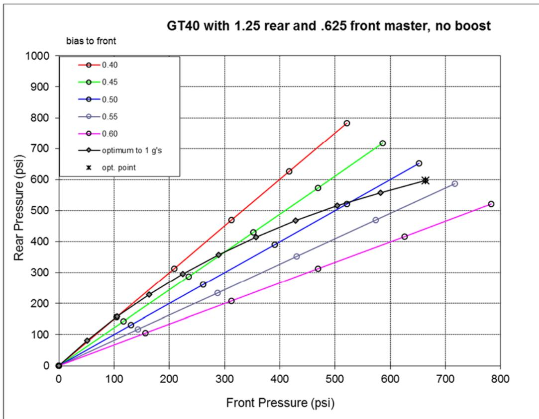
Notice now that I get 1 g's of braking with 100 pounds of foot force with a bias bar setting close to 50%. With this setup I could lock the tires, but it still took a lot of force from the foot. On the track, I don't want to have to hit the brakes that hard quickly. So my next step was to replace the pads.
