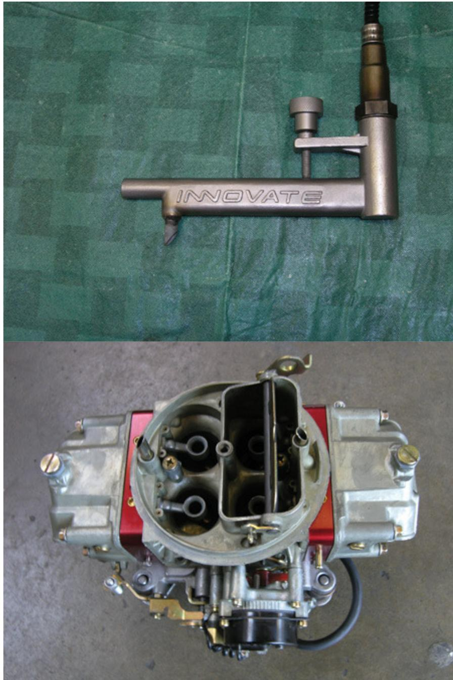
Top: This Unique Innovate tailpipe probe allows you to read the air/fuel mixture without welding a bung into the exhaust system.
