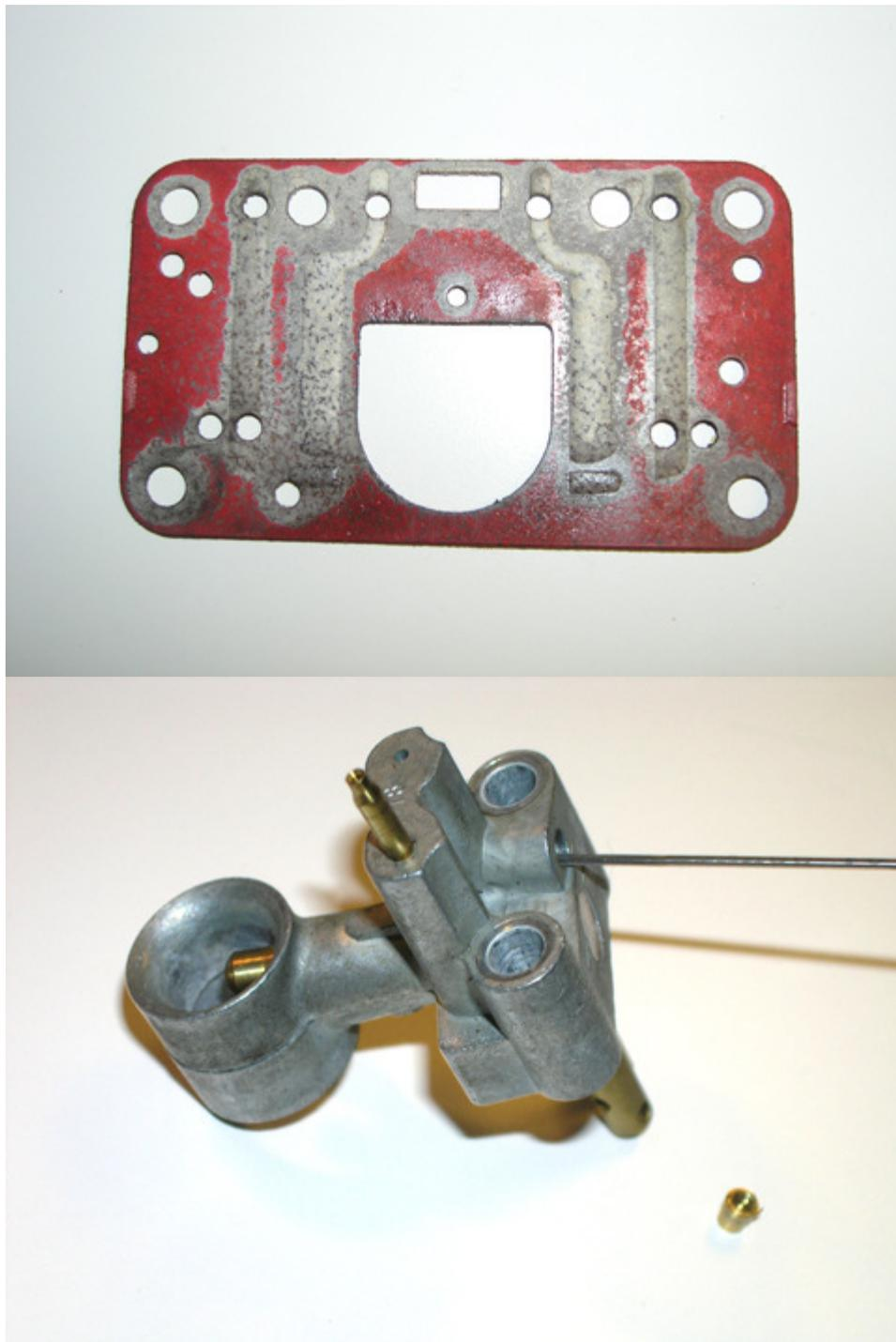
Top: The discoloration of this gasket from a modular carburetor is evidence of fuel leakage between the carburetor's fuel circuits. This leakage could have been prevented by tightening the fuel bowl screws every 3,000 miles or so.
