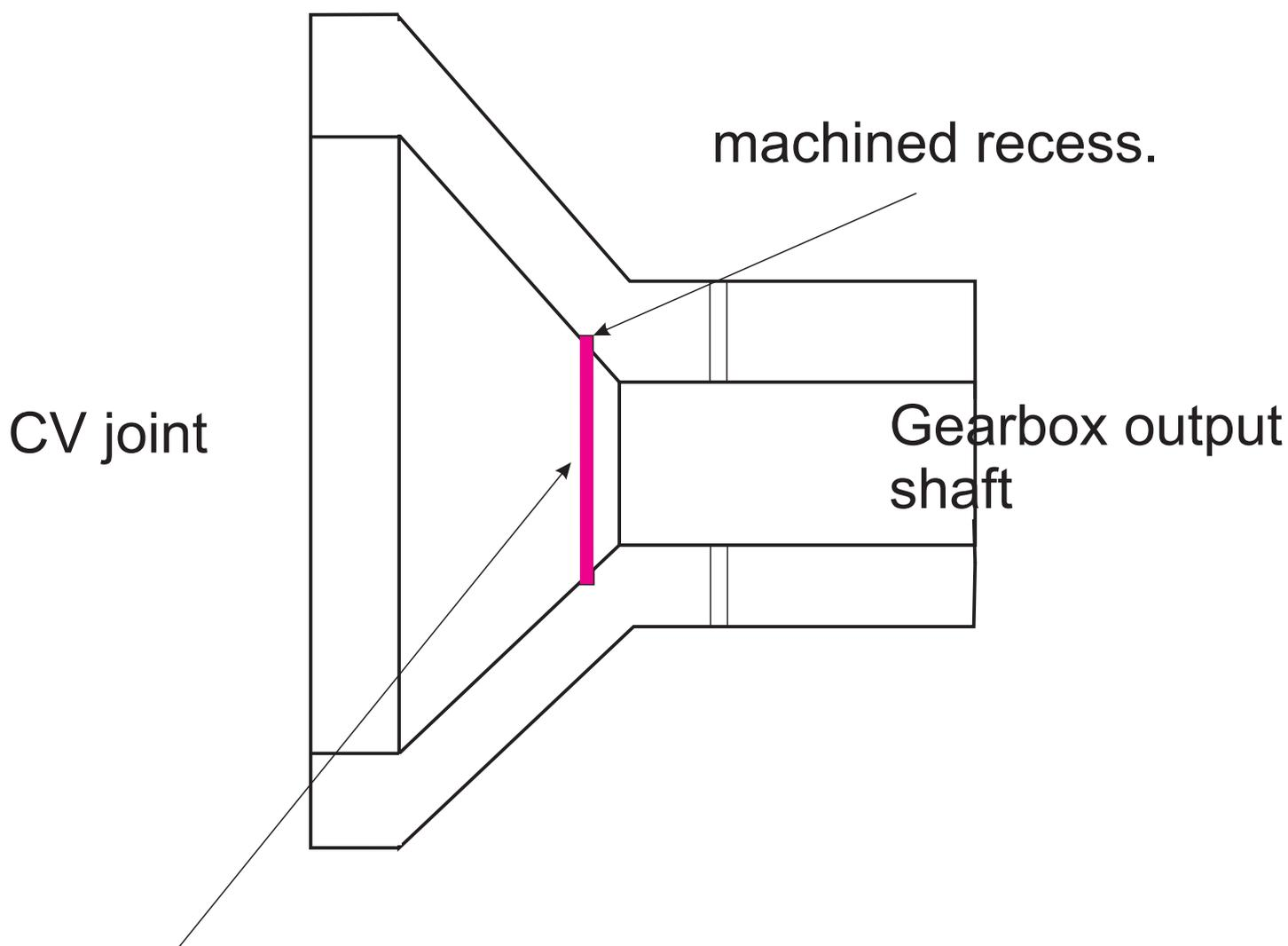
45mm diameter, 2-3mm thick steel disc pressed into recess with interference fit.
