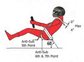
ALWAYS INSPECT THE SEATBELTS BEFORE USE, REPLACE THE WEBBING EVERY TWO YEARS BY RETURNING TO DJ SAFETY.
