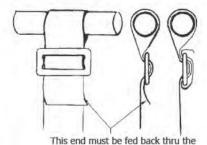
Threading of wrap around style connection. This method can be used around roll bar or frame rails.
