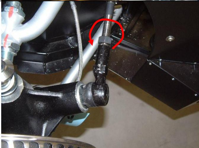
ONCE THE NUT IS REMOVED, REMOVE THE SHAFT OF THE TIE-ROD END OUT THE UPRIGHT. THEN REMOVE THE TIE-ROD END FROM THE STEERING RACK BY TURNING IT ANTI-CLOCKWISE.
