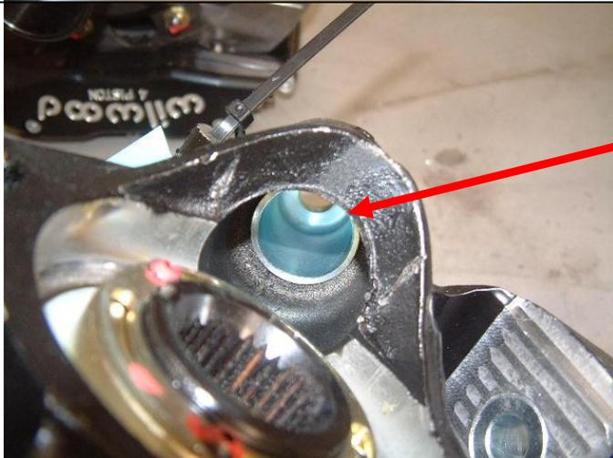
THE NUT THAT SECURES THE TIE-ROD END TO THE UPRIGHT WILL BE VISIBLE HERE.
