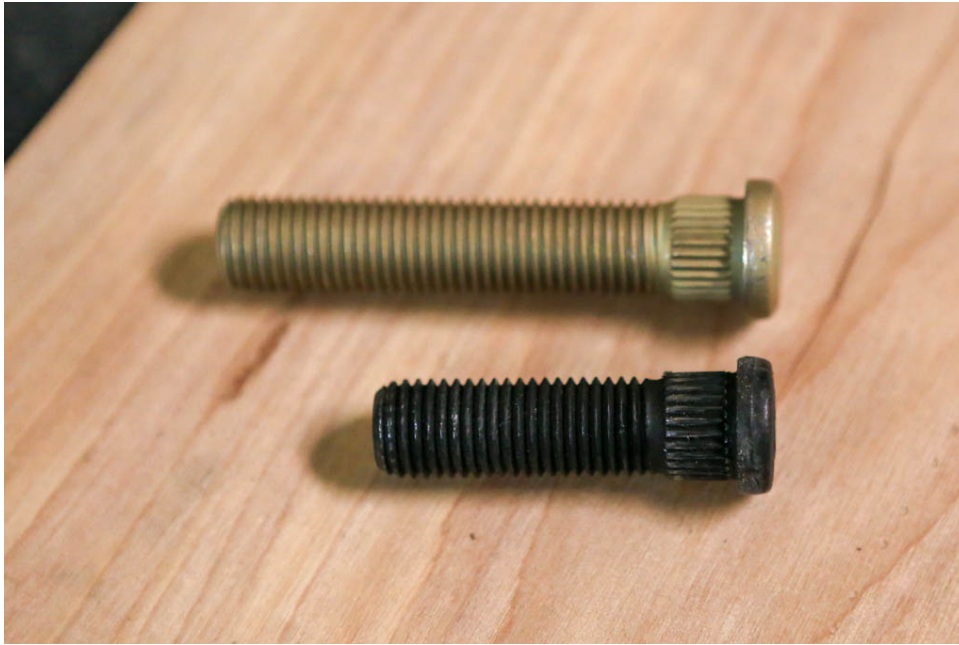
Figure 12: Stud Length Difference
