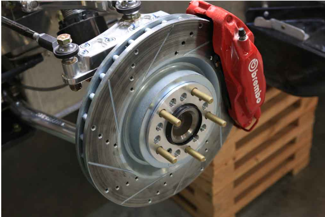
Figure 14: Studs and ¼" Wheel Spacer
