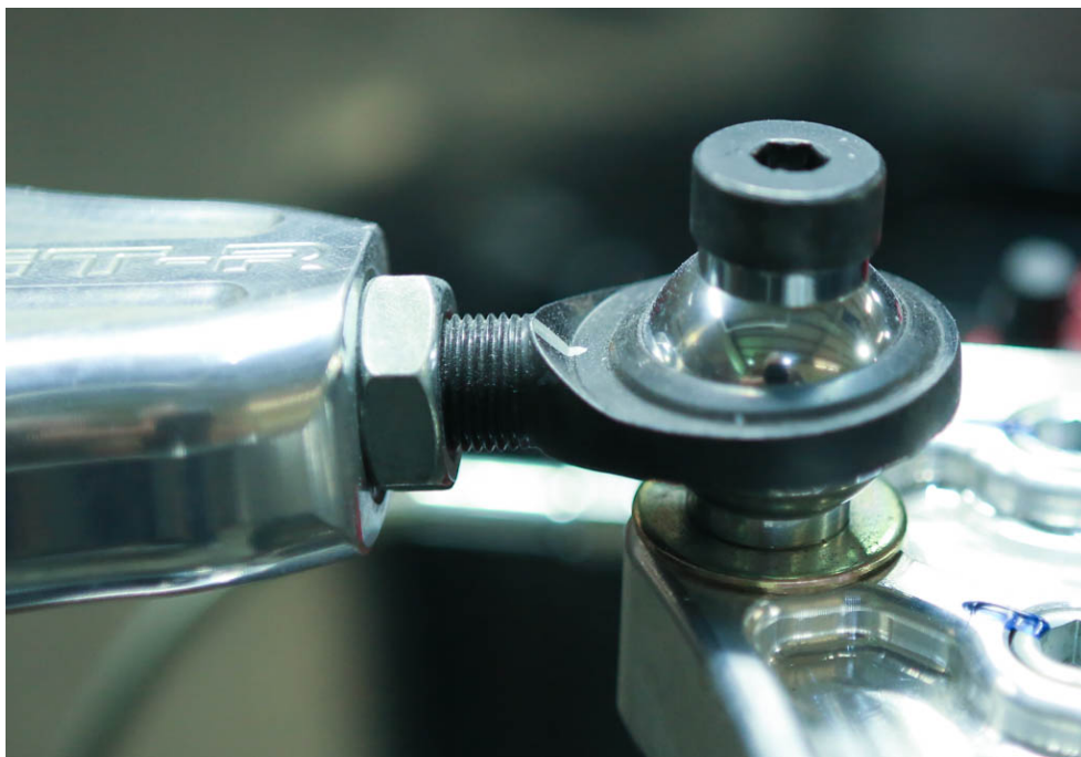
Figure 15: Upper Outboard Rod End
