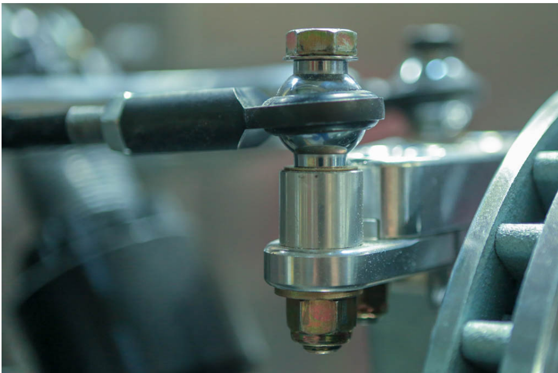
Photo 11: Steering Tie Rod End w/Shortened Standoff
