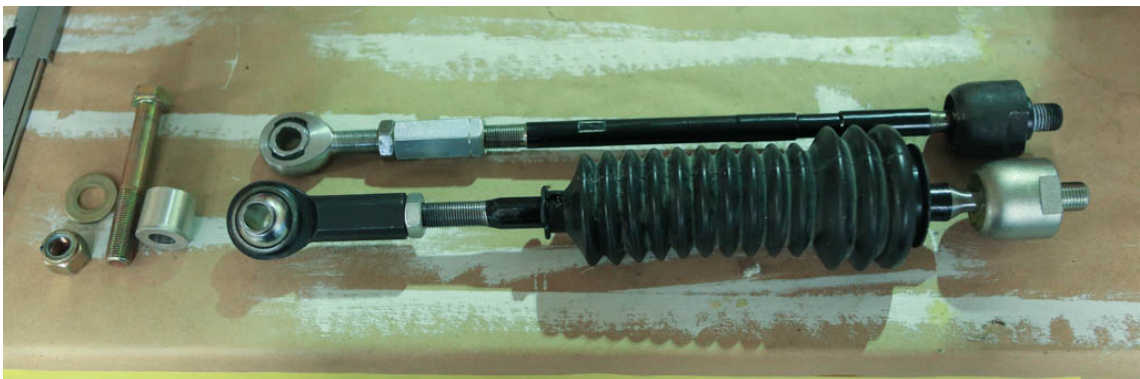
Photo 10: After New Tie Rod Modification
