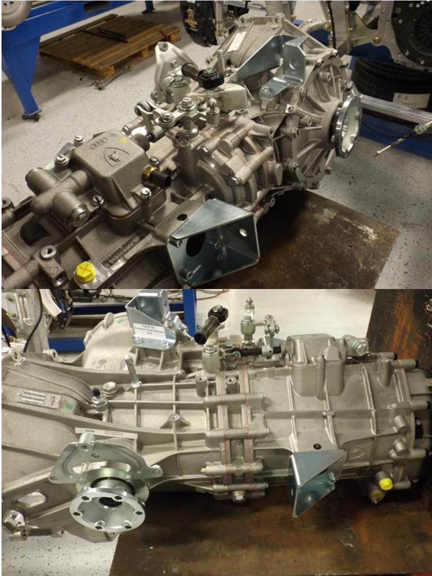
Side mount brackets installed with hole facing forward
