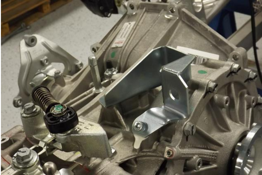
Cable shift bracket installed ontop of transaxle
