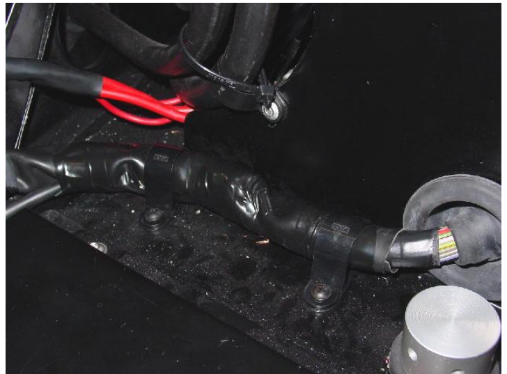
Fig. 14 Reinstall Clamps
