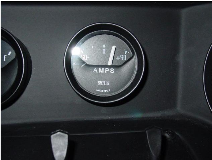
Fig.15 Amp Gauge Connected Backwards
