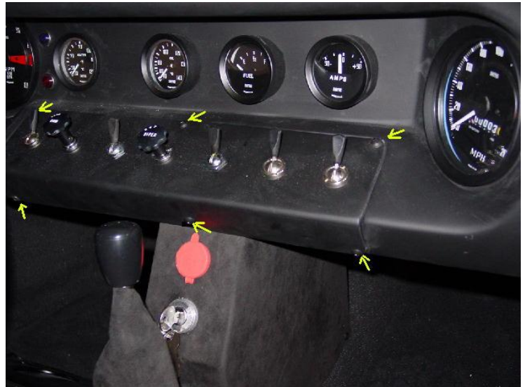
Fig. 16 Screws Location For Panel Removal
