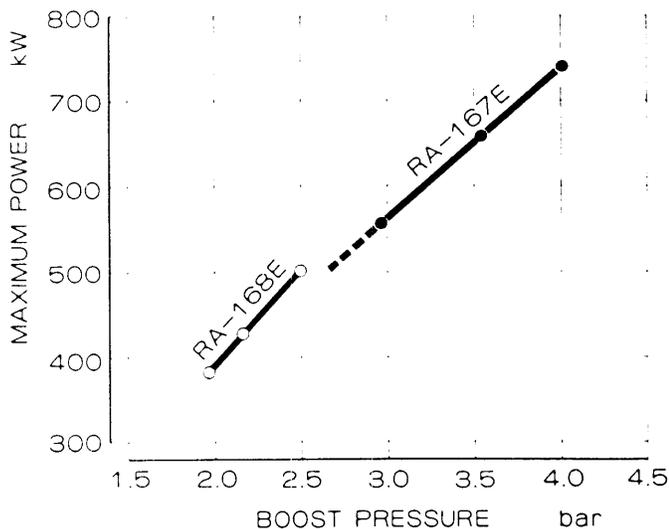
Fig. 5 Maximum power of RA168E and RA167E related to boost pressure
