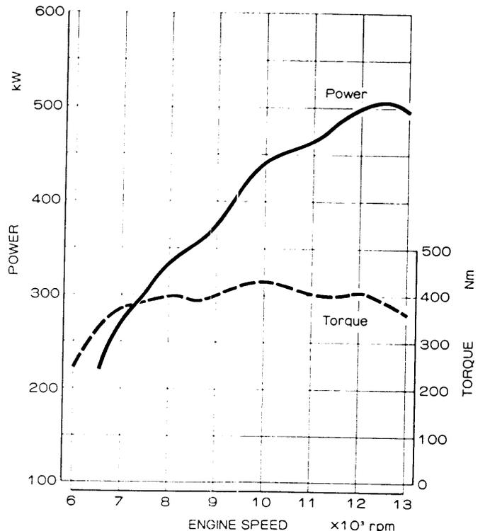
Fig. 4 RA168E power characteristics
