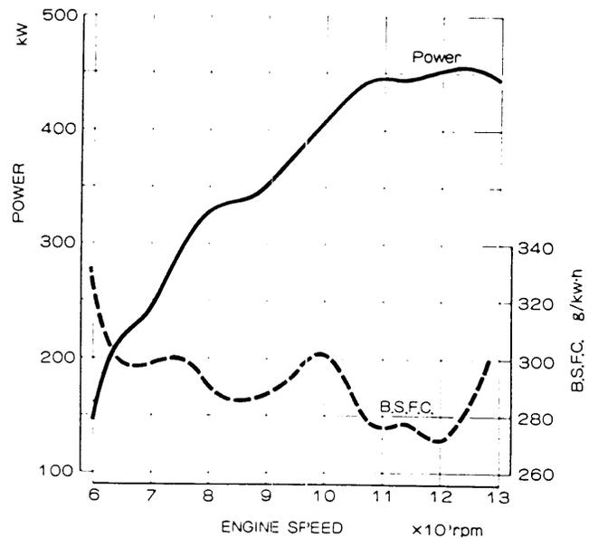
Fig. 9 RA168E performance at minimum fuel consumption
