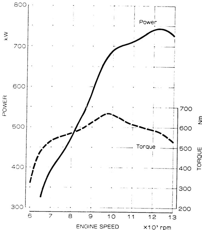
Fig. 3 RA167E power characteristics
