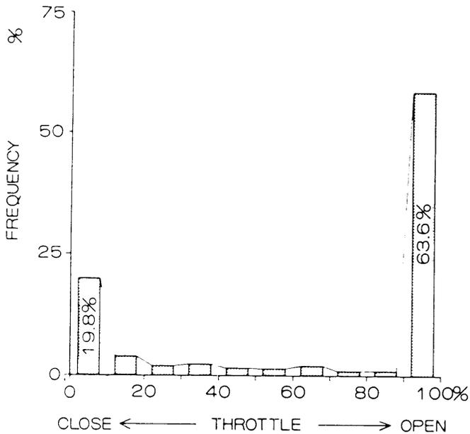
Fig. 8 Throttle opening distribution during a race event ('88 San Marino GP)
