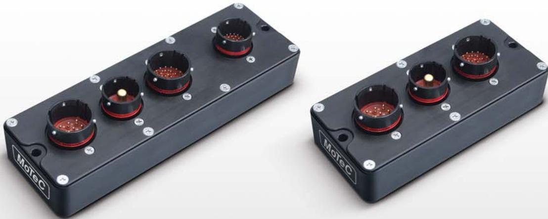
**MoTeC's** new **PDM16** and **PDM32 Power Distribution Modules** replace conventional relays, fuses and circuit breakers by providing electronically switched power to the various electrical systems in the vehicle, including motors, lights, solenoids and electronic devices such as ECUs and data systems. This simplifies wiring and switch requirements, while increasing reliability.
