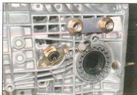
Oil Cooling connections on UN1
