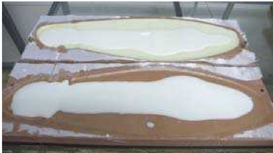
Casting of PB in the two half moulds while the resin film is still liquid
