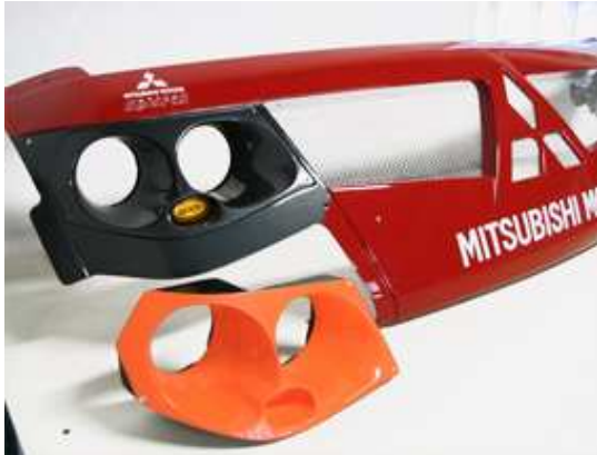
Front light of Paris/Dakar 4 wheel drive Epoxy gel coat and PB 250
