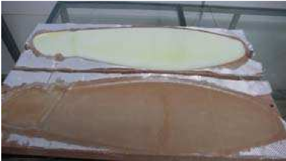
Laminates primed with fast epoxy system
