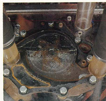
RIGHT: Here's another problem with pumps. When they stop, the coolant level in them can drop, as has happened in this photograph. This can be due to steam pressure and can cause your pump to stall. When the engine is restarted, the pump may be unable to work properly because of the condition.
