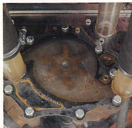
RIGHT: Different speeds have different effects. This doesn't look nearly as bad as the previous shot. Nonetheless, it's still far worse than it should be and will lead to overheating.
