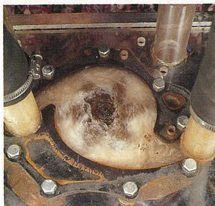
LEFT: Here's a standard Cleveland pump creating really wild cavitation. Note the extreme low-pressure region at the centre of the pressed steel plate impeller.
