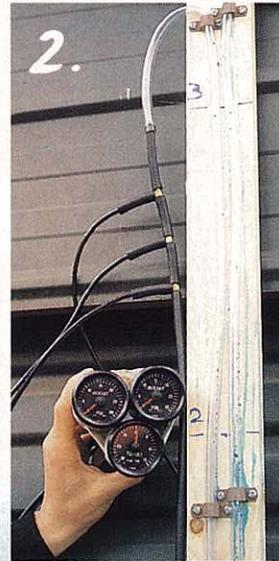
water makes an extremely accurate measuring device called a manometer. When there is no pressure in the tube, the water levels in each side will be level with each other. As pressure in the side with the gauges is increased, water in the far (open) side of the tube is pushed up. It takes 1psi to create a difference of 27 inches between the levels of water in either side of the tube. So when the pressure side drops 13.5" and the open side rises 13.5" (a difference
