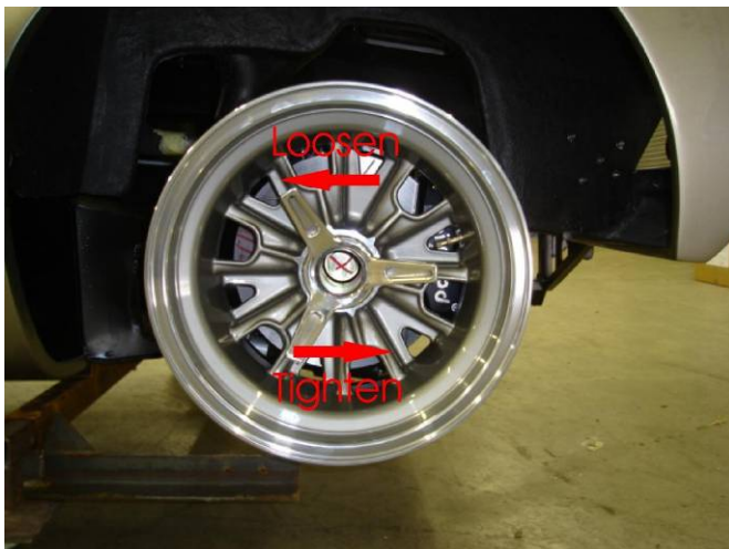
[Figure 16 – The left side front and rear wheel spinners are loosened by turning them counterclockwise and tightened by turning them clockwise.]
