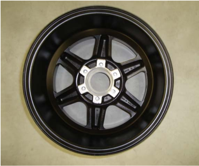
[Figure 18 - Drive Pin Holes in Wheel Centre]
